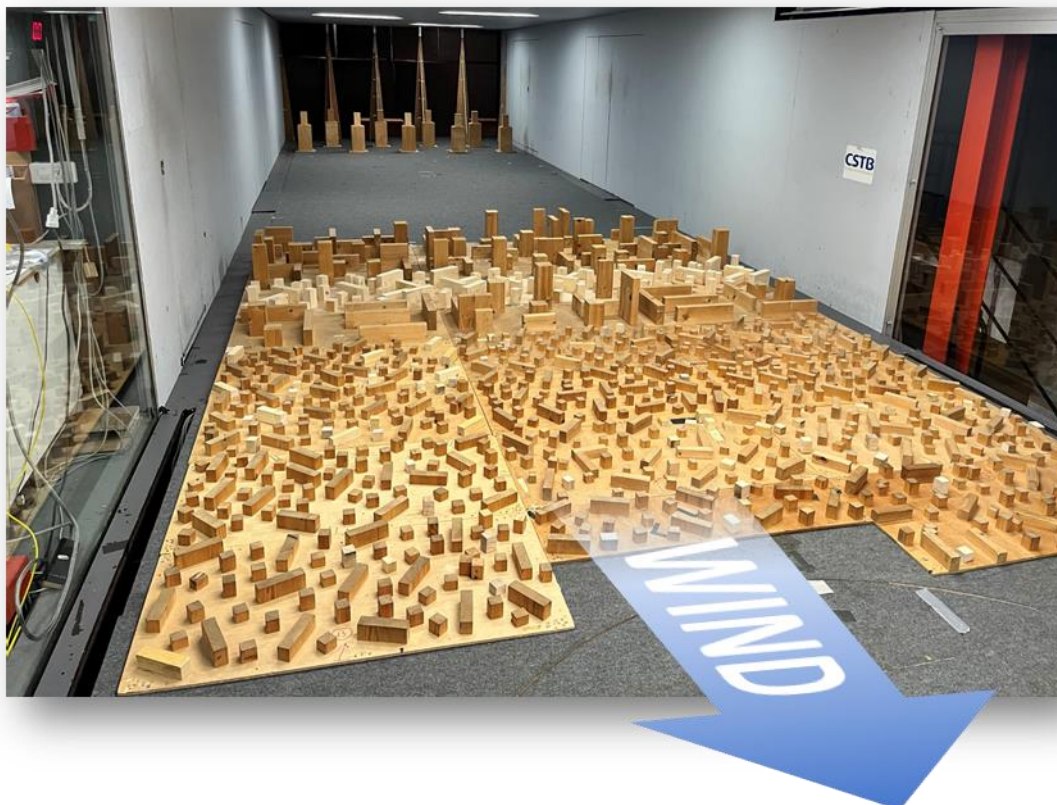
Figure 26 - Roughness upstream of the model
