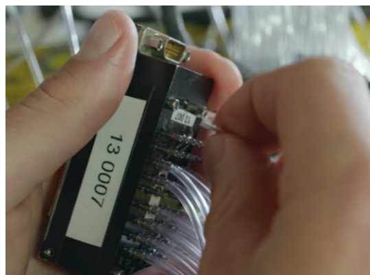
Figure 31 - 32-channel PSI pressure sensor
