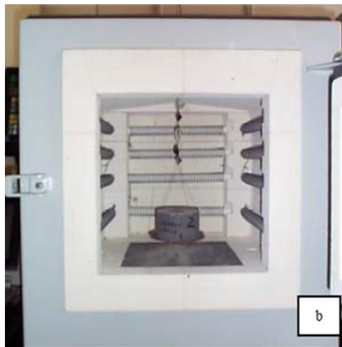
Figure 4: Setup for experimental measurement of the loss of mass in transient heating.
