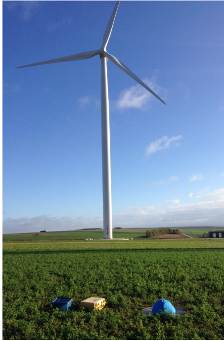
Figure 1: View of one of the measurement point upwind of the wind turbine. The microphone is placed on a hard 1 m diameter board and protected by a windscreen according to IEC 61400 specifications.
