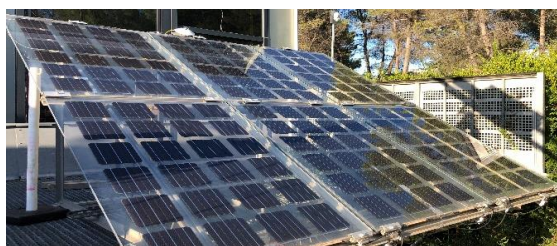
Figure 5 : Canopy mockup on CSTB plateformes – Onyx Solar® modules in BIPVBOOST project – 0,9 kWc.
