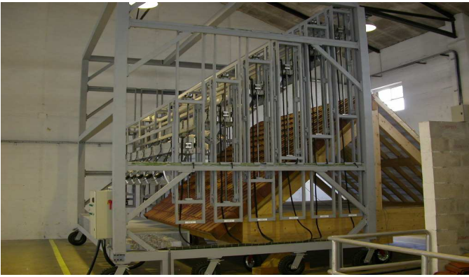
Figure 1. The 3C apparatus; 42 projectors to ensure the solar source radiation; a 45° angle pitched roof can be easily mounted with different systems inside.
