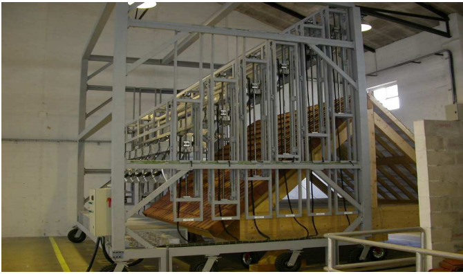
Figure 1. The 3C apparatus; 42 projectors to ensure the solar source radiation; a 45° angle pitched roof can be easily mounted with different systems inside.
