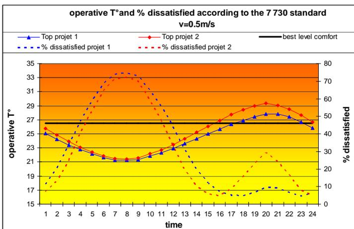
Figure 15: dissatisfied people percentage in an attic with two different roof solar factors with a 0.5 air velocity.
