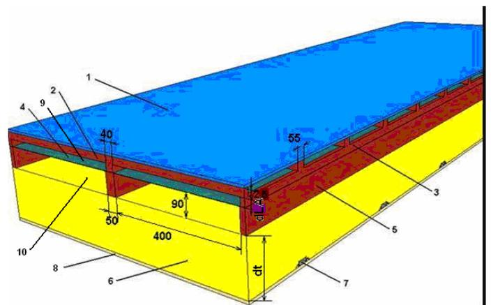
Figure 4: 1 - Tiles ; 2 – battens ; 3 - Laths ; 4 – high vapor permeability wind barrier; 5 – rafters; 6 – Glass wool; 7 – steel studs ; 8 – Gypsum board ; 9 – ventilated air gap; 10 – unventilated air gap.
