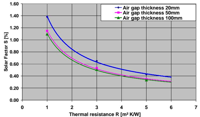
Figure 7:  $S$  function of thermal resistance for various ventilated air gap thickness with a wind barrier emissivity  $\epsilon=0.6$ .
