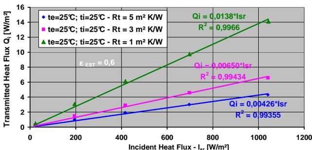
Figure 6.  $Q_i$  (solar factor  $S$ ) function of the thermal resistance.
