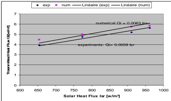
Figure 5: experimental and numerical comparison of solar factor;  $Q_i$  function of the incident heat flux radiation; solid line: experiments; dashed line: simulations.
