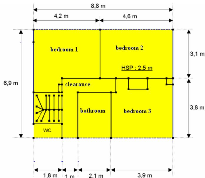
Figure 11: attic main geometrical characteristics
