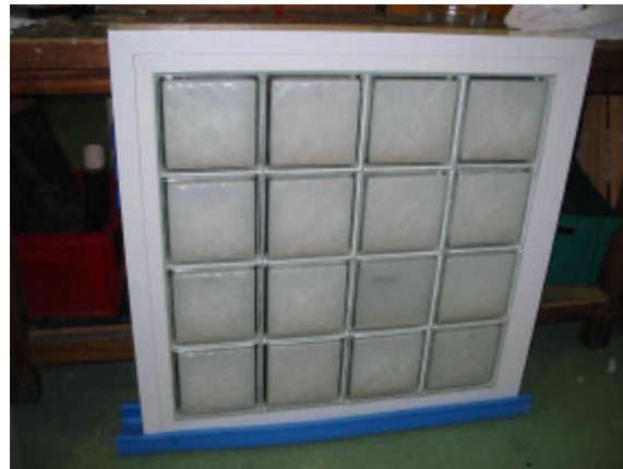
Figure 2: Glass bricks wall containing PCM
