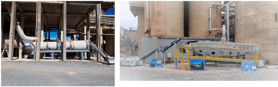
Fig. 7. The two dynamic systems. On the left, the rolling drum carbonator (Créchy cement works) and, on the right, the fluidized bed carbonator (Val d'Azergues cement works).
