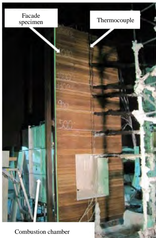
Figure 3: Outline of equipment, (JIS A 1310 facade test).
