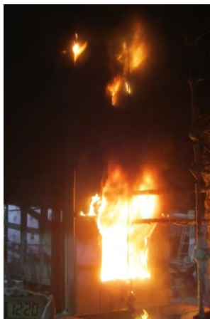
Fig. 4 Specimen of only main façade, during JIS A 1310 test
