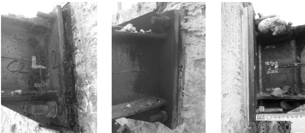
Fig. 8. Thermal breaks after test (left to right: configurations 2, 3 and 4)
