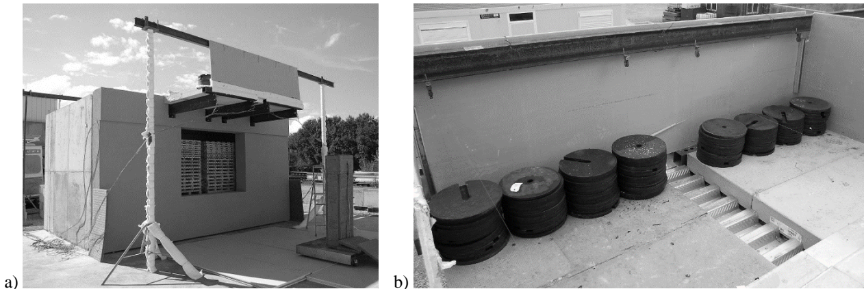
Fig. 5. a) Complete test setup; b) Slab loaded
