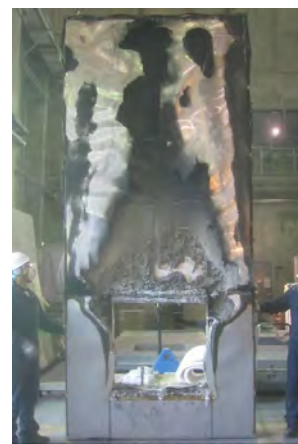
Fig. 5 Specimen of only main façade, after JIS A 1310 test
