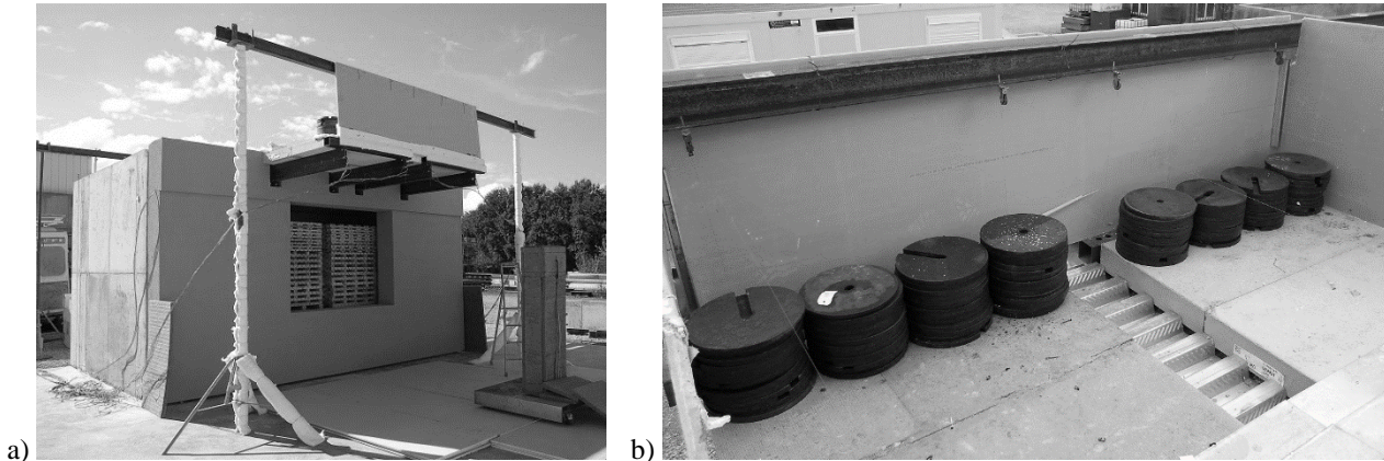
Fig. 5. a) Complete test setup; b) Slab loaded
