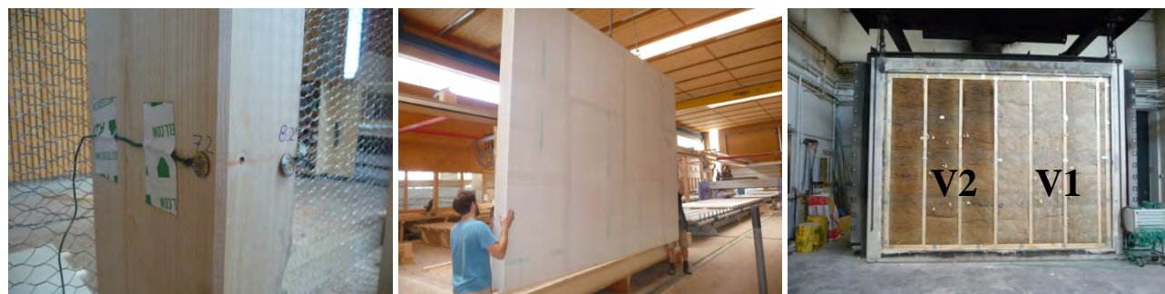
Fig. 3. a) arrangement of thermocouples; b) specimen ready for transport; c) specimen after 90 min testing
