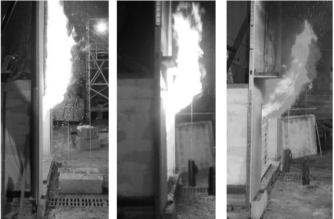
Figure 1 Pictures of flames at the façade without a deflector (left) [1,2], with a 10 cm deflector (middle) and with a 30 cm deflector (right)
