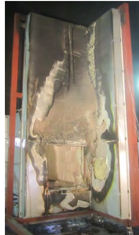
Fig. 7 Specimen with wing façade, after JIS A 1310 test
