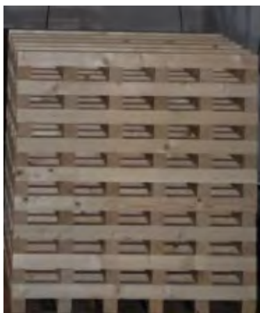
Figure 3 Picture of the wood crib used in the tests and averaged value of HRR calculated from the mass loss rate
