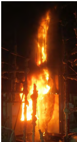
Fig. 6 Specimen with wing façade, during JIS A 1310 test (around 10 min).
