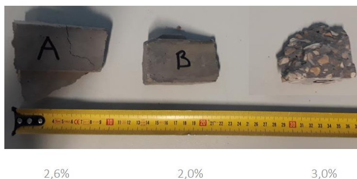
Figure 2: Water content of concrete pieces detached from the segment corners
