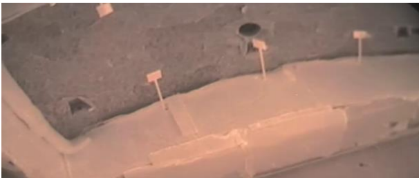
Figure 24: Segment in the furnace during the fire test after 8 min taken with one of the 2 endoscopes
