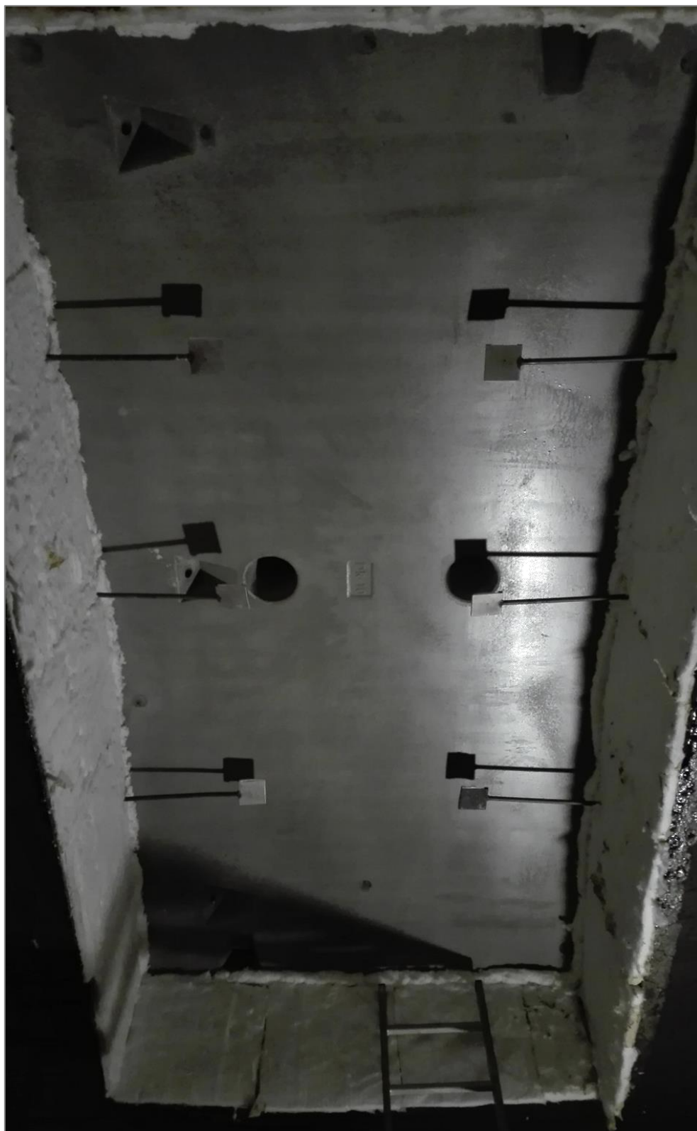
Figure 17: View in the furnace of a single segment after applying thermal protection
