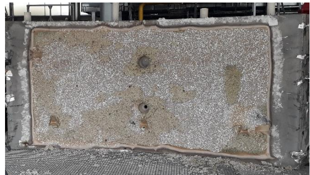
Figure 27: Segment 2 hour after being removed from the furnace during the 3D laser scanning
