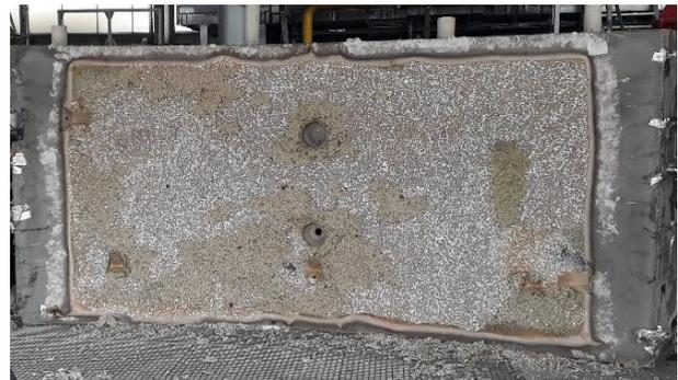
Figure 27: Segment 2 hour after being removed from the furnace during the 3D laser scanning
