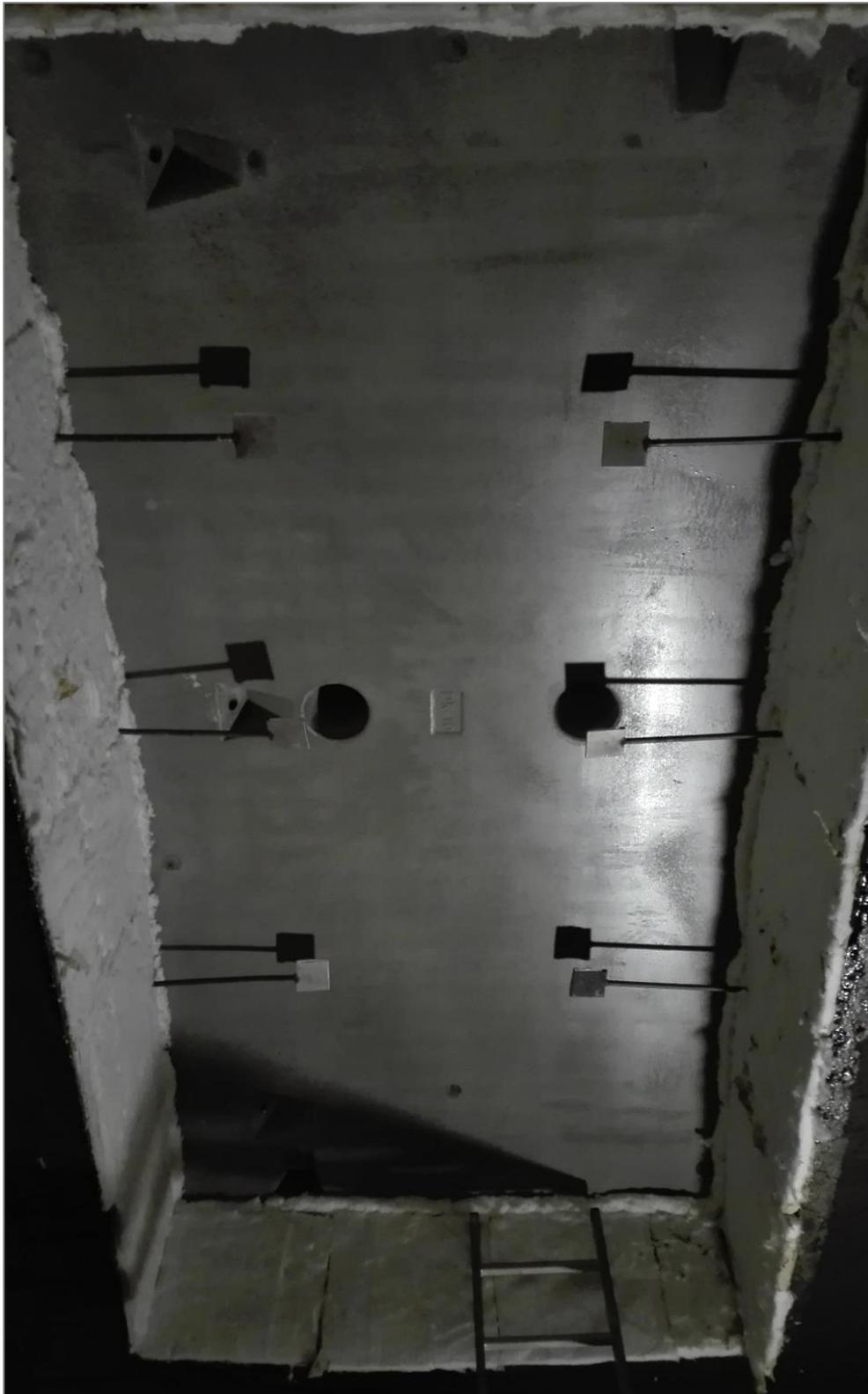
Figure 17: View in the furnace of a single segment after applying thermal protection
