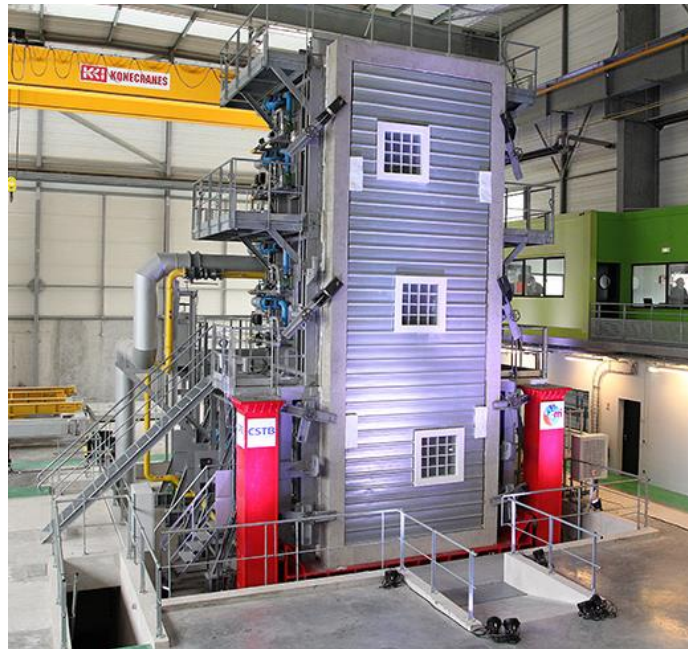
Fig.3 : Vulcain furnace of CSTB Champs-sur-Marne, France
