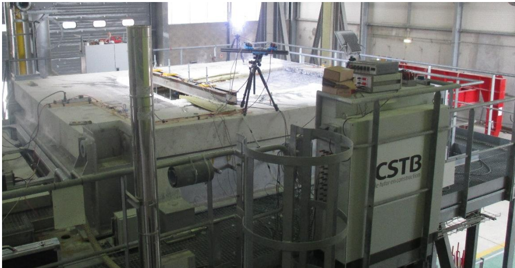
Fig. 15: Full-scale fire test on a concrete cantilever slab connected to a concrete wall by chemical anchors performed on the Vulcain furnace (CSTB, Champs-sur-Marne, France)
