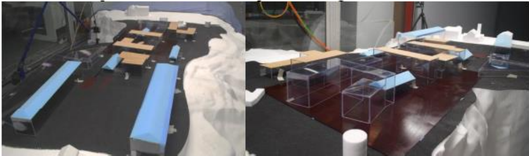
Figure 6 - Model of the district for wind tunnel experiments
