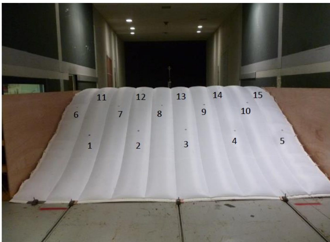
Figure 14: Location of displacement measurement targets on the fabrics.
