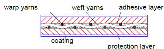
Figure 6: structure of a coated fabric
