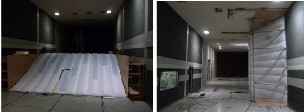
Figure 10: Model of inflatable convergent in the high speed section of the wind tunnel, in horizontal and vertical location
