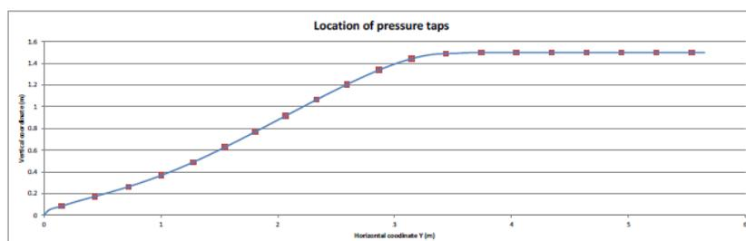
Figure 11: Shape of the inflatable convergent model at rest and location of pressure taps
