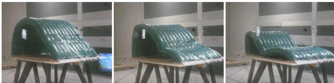
Figure 5: experiments with inflated structures inside the Jules Verne wind tunnel, studying its collapsing with wind
