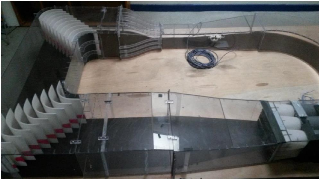
Figure 5: Model of the future wind tunnel made of transparent material in order to enable PIV measurements
