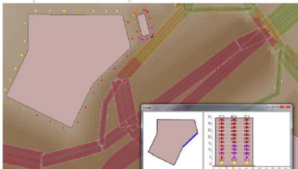
Figure 7: Example of building facade noise level calculation (same color code as above)
