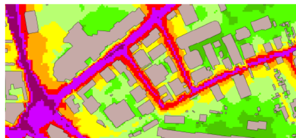
Figure 6: Generated L_{den} horizontal noise map. dB values vary between below 45 (deep green) to above 75 (deep purple).
