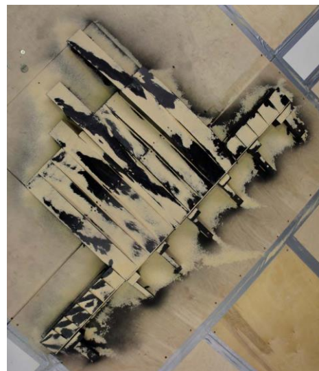
Figure 8. Typical areas of snow deposits, the angle of the incoming flow is 45^\circ
