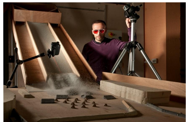
Figure 12. Small-scale physical model of the runout zone fed with granular flows from a channel of adjustable slope and equipped with a reservoir at the top to release granular material
