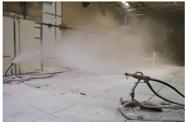
Figure 2. Snow guns in operation in the thermal circuit of the Jules Verne CWT
