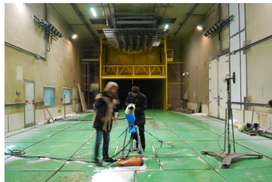
Figure 12. Setting of the CPI Particle imaging probe
