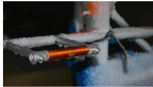
Figure 19. Early version of the LW hot wire snow probe.
