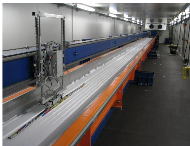
Figure 1. The linear tribometer of the Department of Sport Science of the University of Innsbruck
