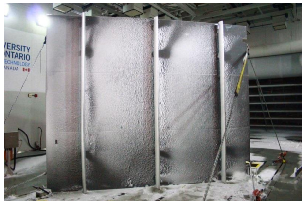
Figure 11. Example of tests in a climatic simulation chamber for wind, snow and ice
