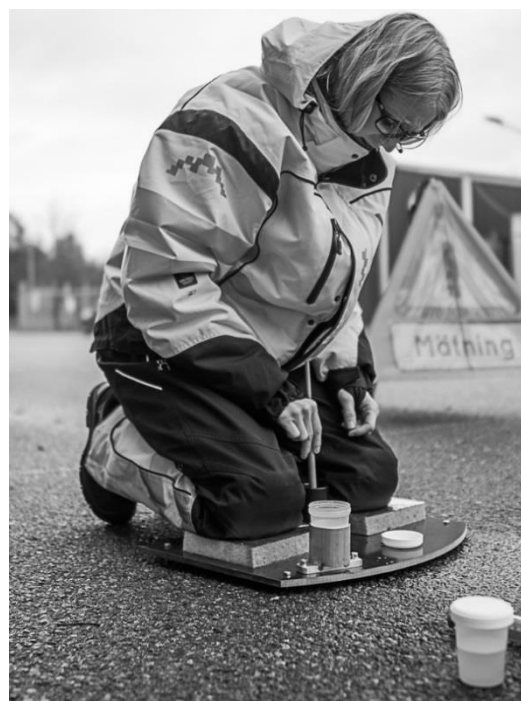
Figure 1. Portable salt measuring and sampling device.
