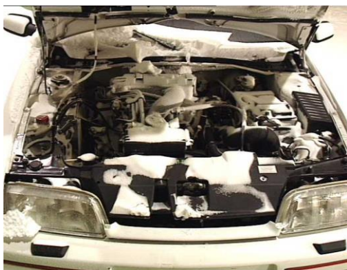
Figure 10. Snow ingress under the bonnet of a road vehicle at the end of a wind tunnel test
