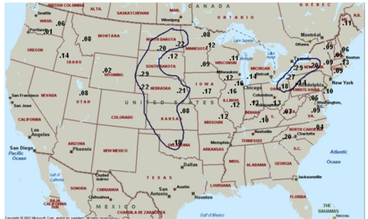
Figure 2. Simulated 50-year drift ratios for upwind fetch L_u = 250 ft.
