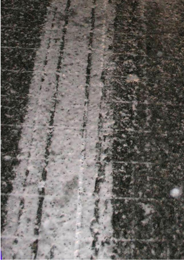
Figure 5. Example of a thin layer of wet snow compressed by a single aircraft tire passage. The runway sweeper was able to remove all loose wet snow, but not the snow compressed by the tire. The longitudinal grooves present in the aircraft tire can be recognized in the track.
