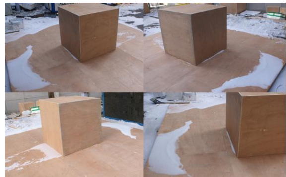
Figure 5(c). Photos of snowdrift with 4.5m/s wind speed
