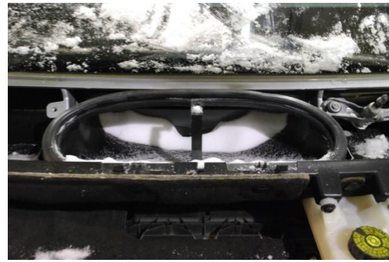
Figure 5. Dry snow ingress in the HVAC air intake of a road vehicle
