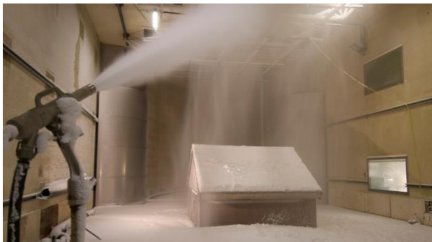
Figure 1. Snow test in a climatic wind tunnel
