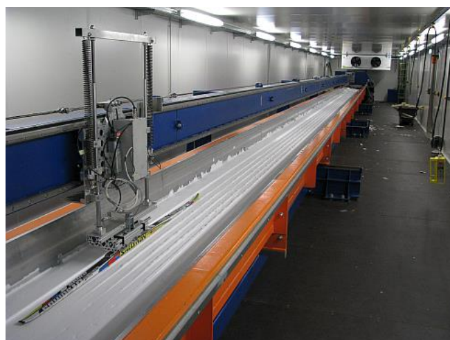
Figure 1. The linear tribometer of the Department of Sport Science of the University of Innsbruck.
