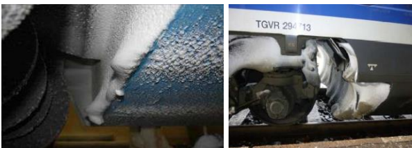
Figure 18: Snow accumulation in the bogie cavity (wind tunnel model and real TGV train)
