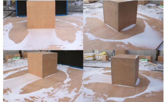
Figure 5(a). Photos of snowdrift with 2.5m/s wind speed
