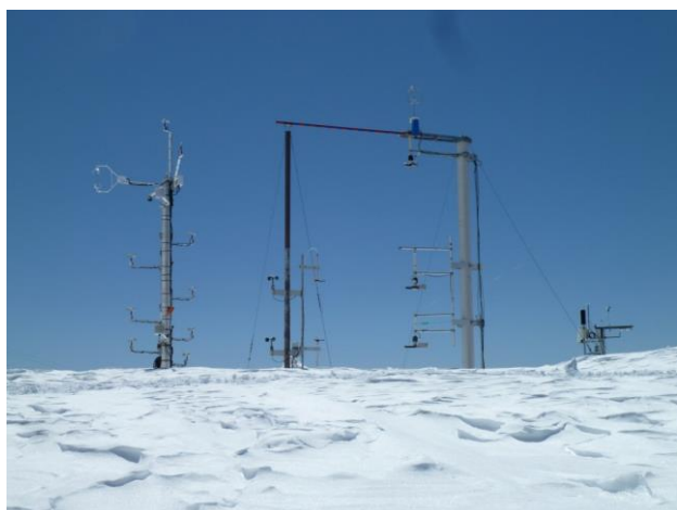
Figure 24. Ultrasonic anemometer, wind anemometer profile, acoustic and optical snow transport sensors
