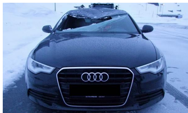
Figure 3. Damaged front shield of a car hit by a falling chunk of snow on San Bernardino national highway, on 1 February 2014 (Photo Kantonspolizei Graubünden).
