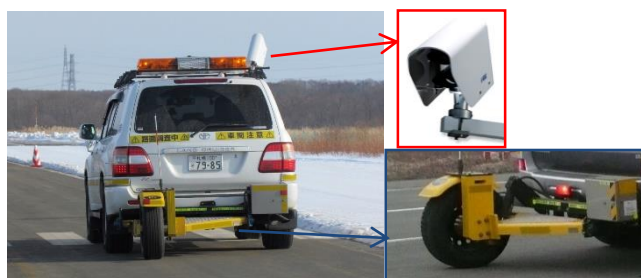
Figure 1. Test vehicle equipped with the CFT and the DSC-111
