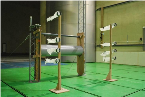
Figure 4. Measurement of the snow concentration in the airflow by net snow collectors
