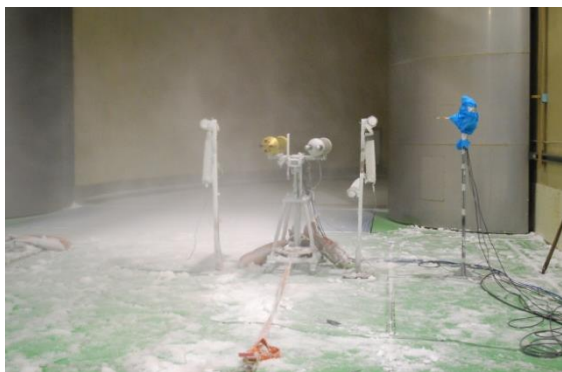
Figure 7. Snow test with the particle imaging probes 2DS
