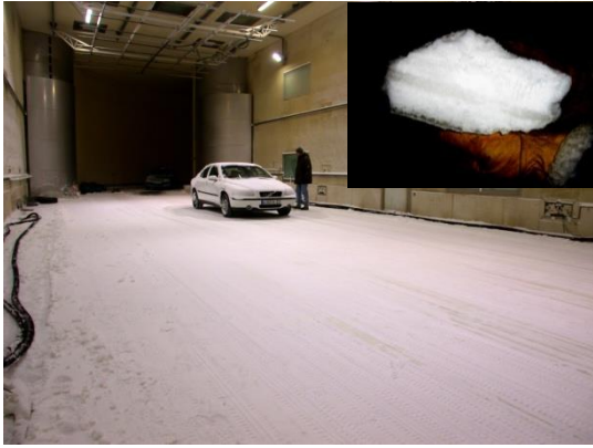
Figure 13. Tyre adherence tests on a stratified and compacted road snow layer in the wind tunnel
