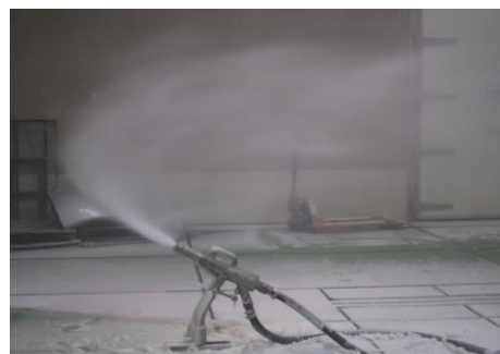
Figure 4. Positioning of snow cannon against the flow in the wind tunnel
