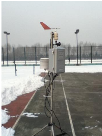
Figure 3. PC-4 automatic weather station
