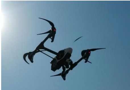
Figure 4. UAV equipped for the purpose of photogrammetric measurement of roof snow depth
