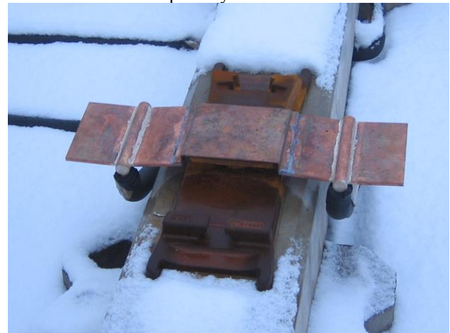
Figure 5. First prototype of the switch point heating system
