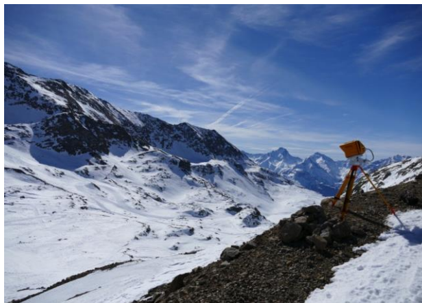
Figure 25. Terrestrial laser scanner and general view of the experimental site.
