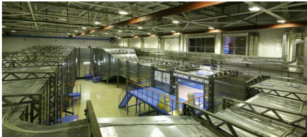
Figure 5. Boundary Layer Wind Tunnel of Moscow State University Of Civil Engineering
