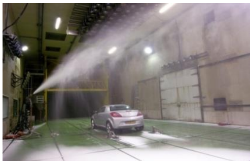
Figure 9. Snow test of vehicles in the wind tunnel
