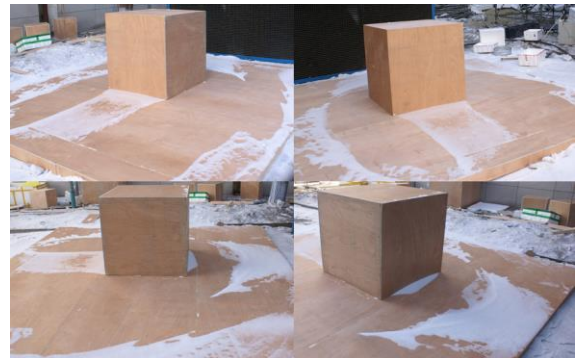
Figure 5(b). Photos of snowdrift with 3.5m/s wind speed
