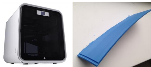
Figure 3. 3D Printer Cube Pro and roofing element.
