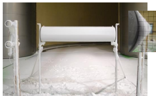
Figure 19. Experimental and numerical modeling of wet snow impact and accretion cylinders of various diameters (diam. 50, 200 and 315mm)
