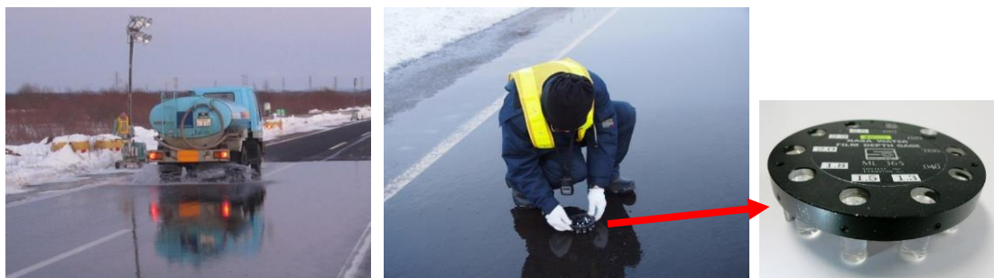
Figure 4. Creation of the wet surfaces (left) and measurement of water thickness with the NASA water-film depth gauge (right).
