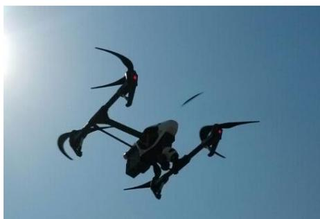
**Figure 4.** UAV equipped for the purpose of photogrammetric measurement of roof snow depth
