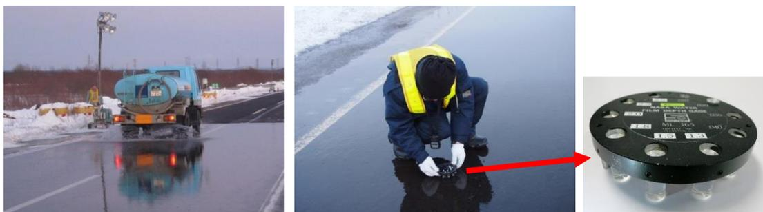
Figure 4. Creation of the wet surfaces (left) and measurement of water thickness with the NASA water-film depth gauge (right).
