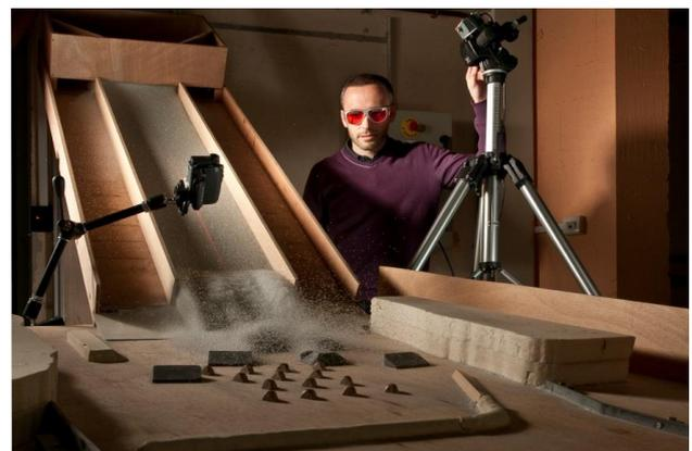
**Figure 12.** Small-scale physical model of the runout zone fed with granular flows from a channel of adjustable slope and equipped with a reservoir at the top to release granular material
