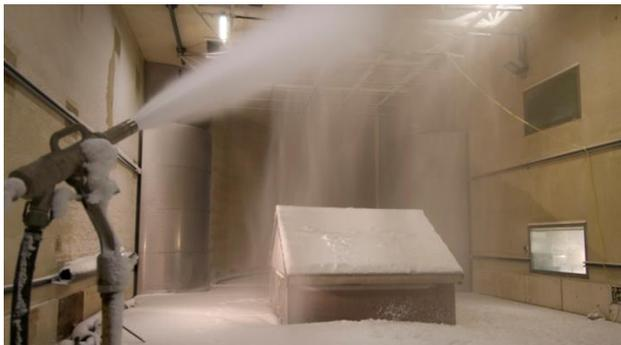
**Figure 1.** Snow test in a climatic wind tunnel
