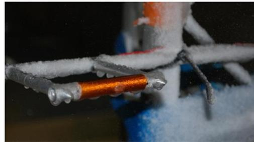
Figure 19. Early version of the LW hot wire snow probe.
