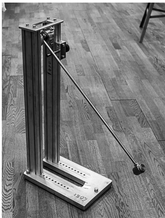
**Figure 3.** Ice quality measuring device.
