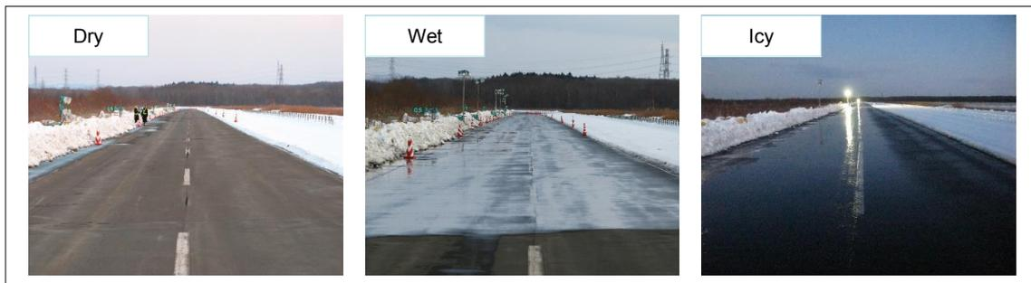
Figure 2. Road surface conditions used for the test.
