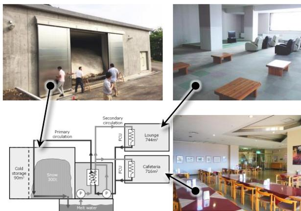
Figure 3. Snow-cooling system for a spa resort.
