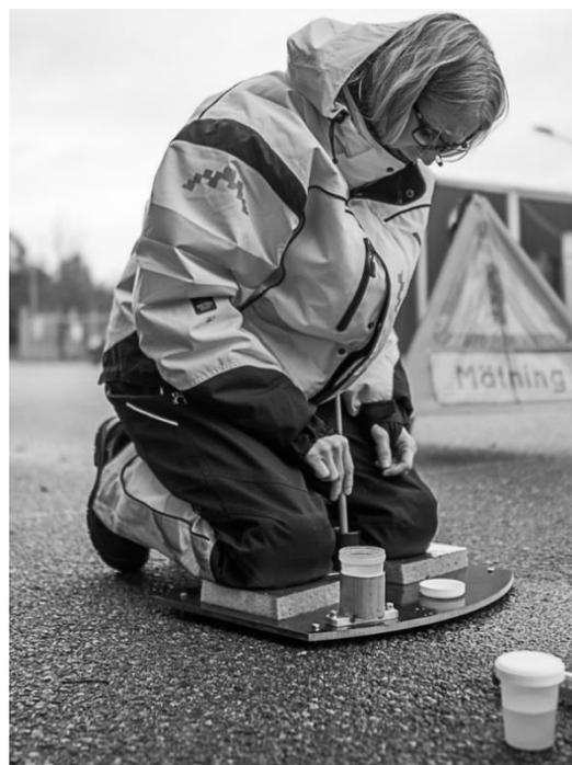
**Figure 1.** Portable salt measuring and sampling device.
