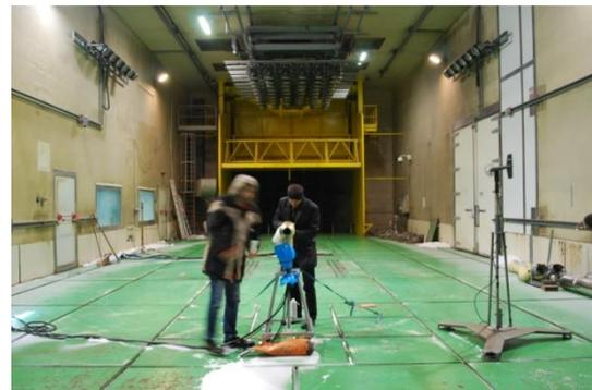
**Figure 12.** Setting of the CPI Particle imaging probe
