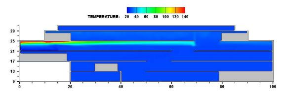
Figure 51: Temperature contour at 1200 s at y=10 m, with the resulting strategy (scenario 29)
