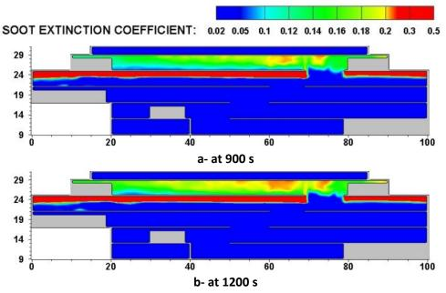
Figure 47: Extinction coefficient contour at y=10 m, with the resulting strategy (scenario 30)
