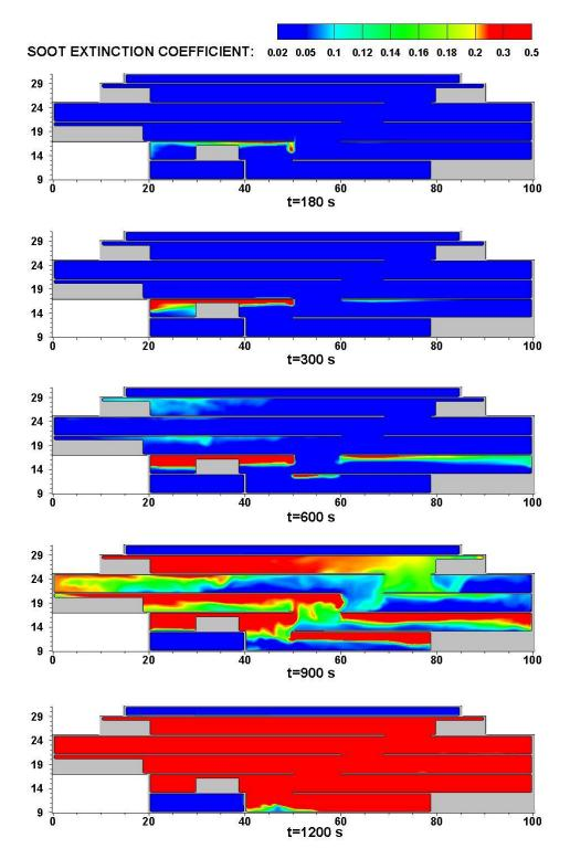
Figure 40: Extinction coefficient contour at given times at y=10 m, with the mechanical smoke exhaust system on the north side on each level (scenario 11)
