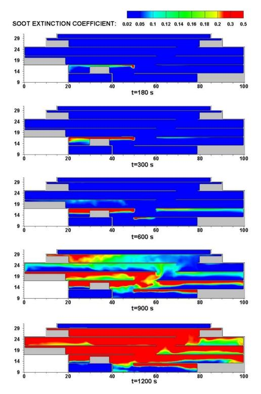
Figure 43: Extinction coefficient contour at given times at y=10 m, with the natural smoke exhaust system and permanent smoke barriers along the edges of floor voids (scenario 12)
