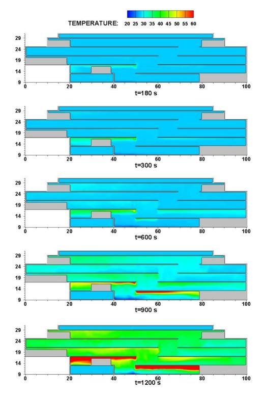
Figure 36: Temperature contour at given times at y=10 m, without smoke exhaust system (scenario 1)
