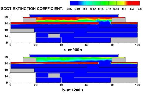
Figure 49: Extinction coefficient contour at y=10 m, with the resulting strategy (scenario 32)
