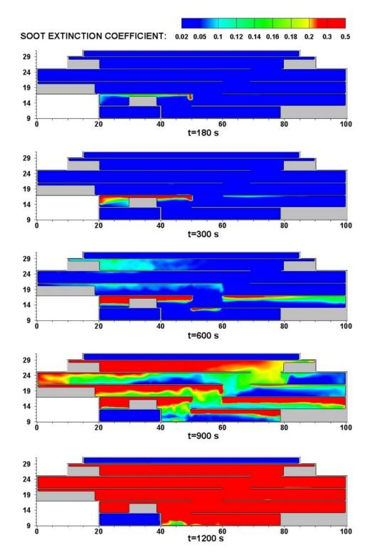
Figure 39: Extinction coefficient contour at given times at y=10 m, with the mechanical smoke exhaust system on the north side on L4 (scenario 8)
