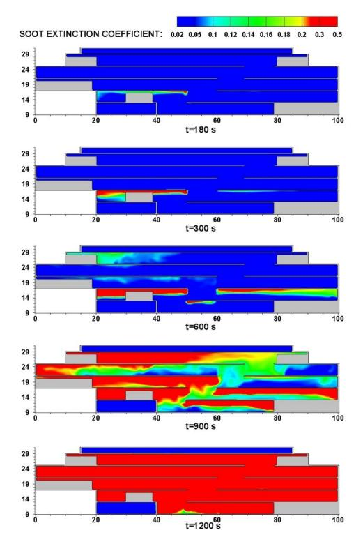
Figure 37: Extinction coefficient contour at given times at y=10 m, without smoke exhaust system (scenario 1)
