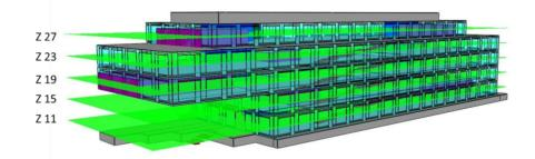
Figure 14 : Horizontal planes for outputs from FDS code
