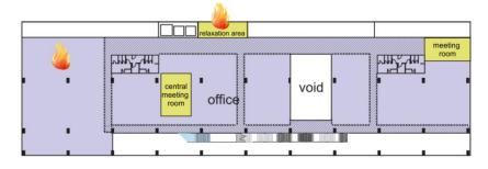
Figure 24: Fire locations on level L7
