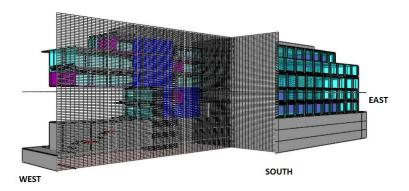
Figure 13 : Building reproduced computationally for FDS calculations
