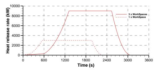
Figure 25: HRR versus time for fires of office furniture (localized and extended)
