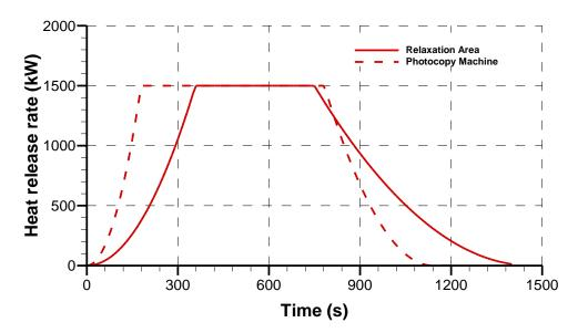
Figure 26: HRR versus time for fire in storage space along floor voids and in relaxation area
