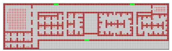
Figure 19: Computational domain for furnished workspaces on level L6
