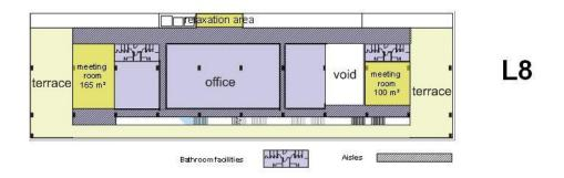
Figure 5: Outline sketch of internal layout on each office level
