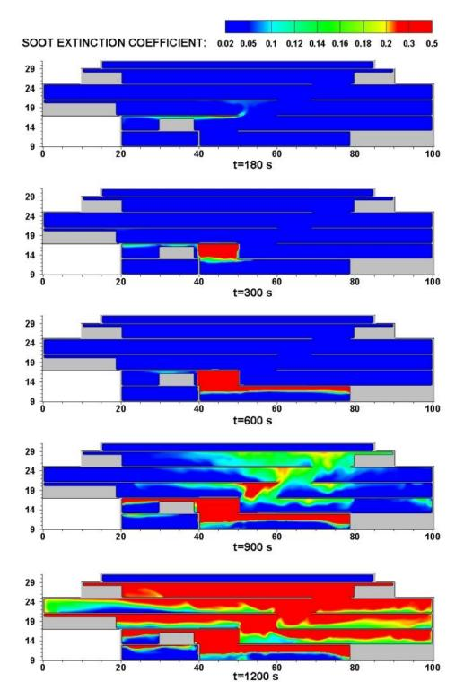
Figure 42: Extinction coefficient contour at given times at y=10 m, with the natural smoke exhaust system and temporary smoke barriers along the edges of floor voids (scenario 13)
