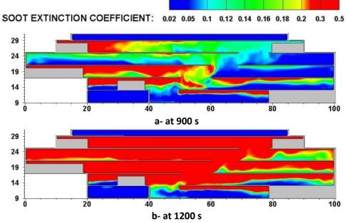
Figure 44: Extinction coefficient contour at y=10 m, with the resulting strategy (scenario 27)
