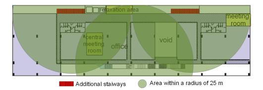
Figure 29: Areas centered on stairway and within a radius of 25 m (example of level L7)
