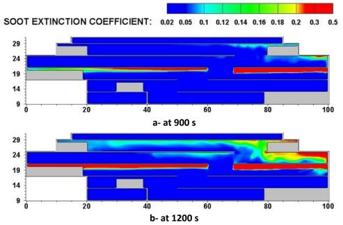
Figure 46: Extinction coefficient contour at y=10 m, with the resulting strategy (scenario 29)
