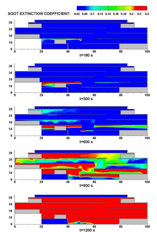
Figure 38: Extinction coefficient contour at given times at y=10 m, with the mechanical smoke exhaust system on the south side (scenario 6)
