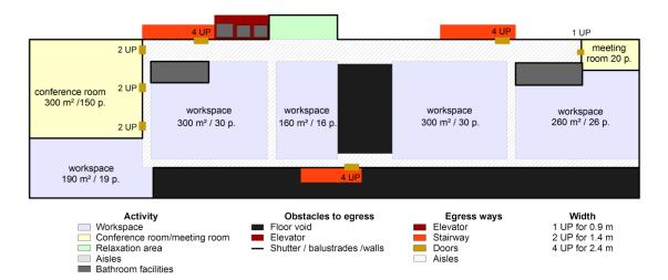
Figure 16: Activity, main obstacles and stairways on level L6
