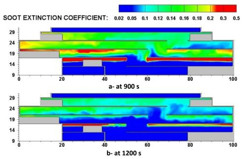
Figure 45: Extinction coefficient contour at y=10 m, with the resulting strategy (scenario 28)
