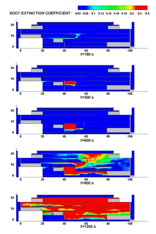
Figure 41: Extinction coefficient contour at given times at y=10 m, with the mechanical smoke exhaust system close to the roof (scenario 16)
